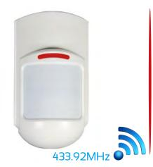
VS-WH400 is top quality wireless PIR motion sensor that adopts dual element infrared sensor for true human movement detection. The sensor with new housing design and using special fresnel lens to reach the high accurate of movement detection. The PIR detector integrated with 433MHz wireless transmitter. When sensor detect the movement, it will send out the signal to alarm systems. With built-in wireless antenna design, the wireless transmission can be up to 100 meters in open space.
